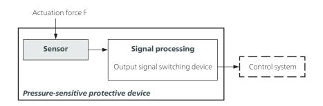
If you combine sensors with control units and thereby place pressure-sensitive protective devices on the market, you should observe the basic requirements according to ISO 13856.
